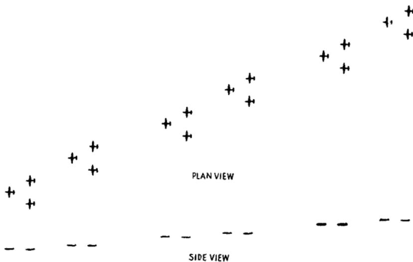
FIGURE 6.—Three-ship V.
