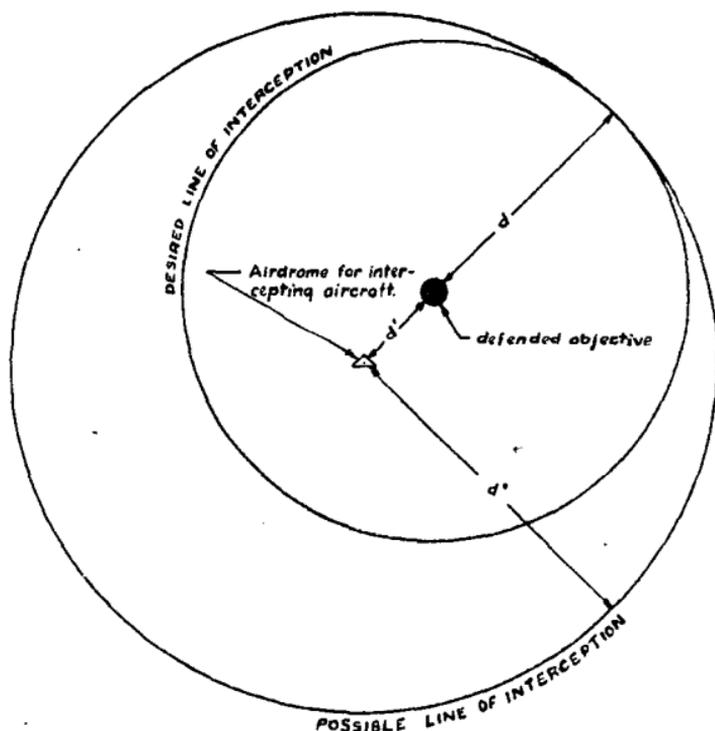
FIGURE 3.—Relation between possible and desired lines of interception.
