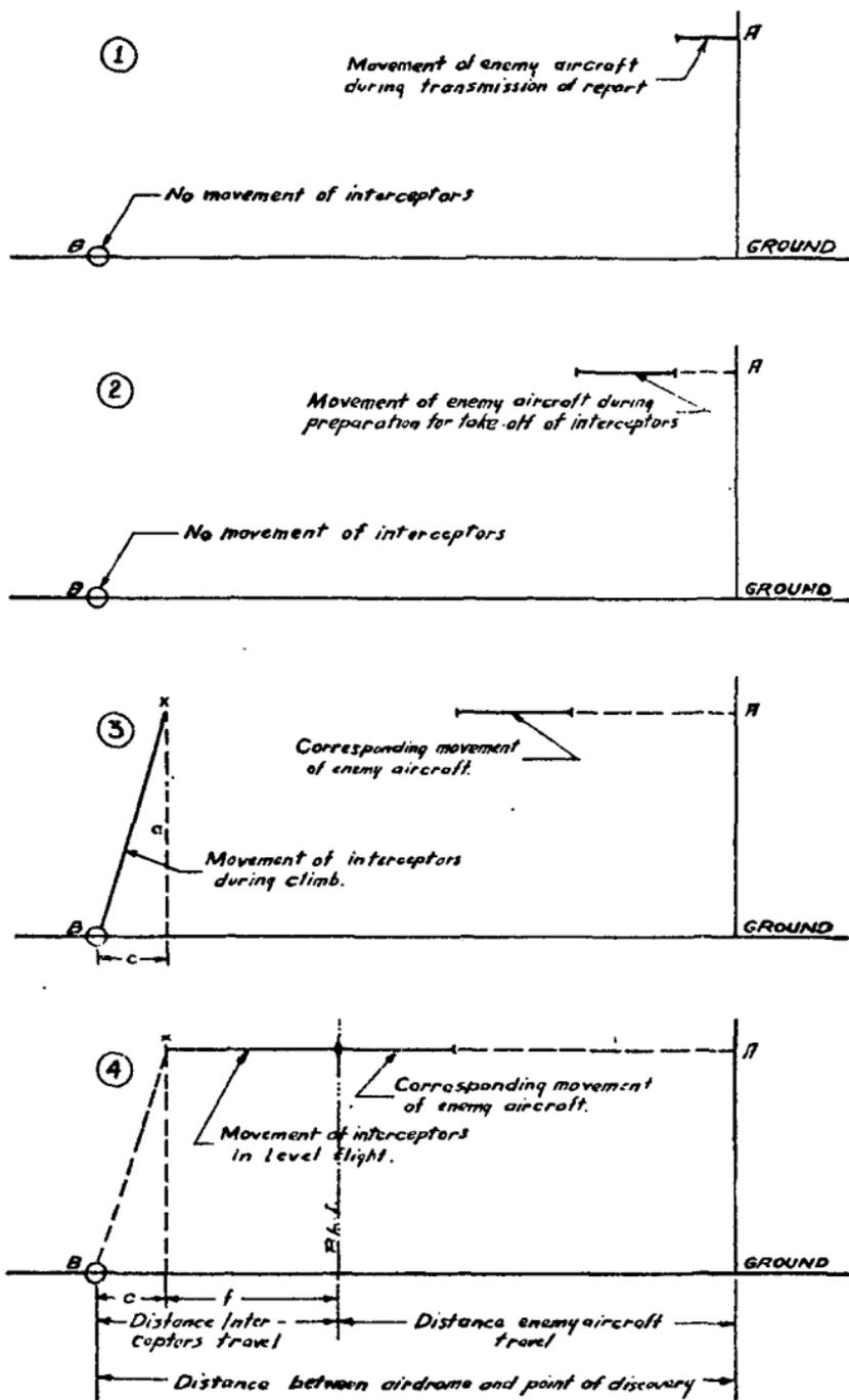
FIGURE 5.—Schematic diagram of interception.
